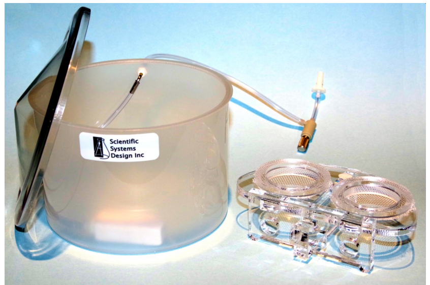
BSK5-2 Brain slice keeper with rings and net in place and with purpose designed container with lid to side. A needle valve is used to control the flow of oxygen mixture to the air-stone.
