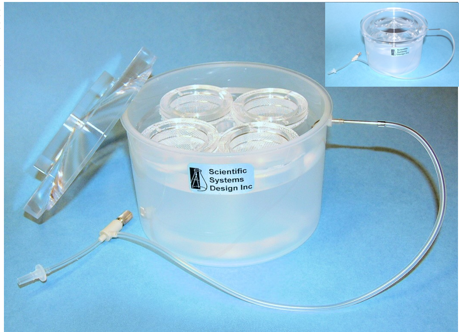
BSK4 Brain slice keeper with rings and net in place and with lid in place (inset). A needle valve is used to control the flow of oxygen mixture to the ceramic bubbler.
