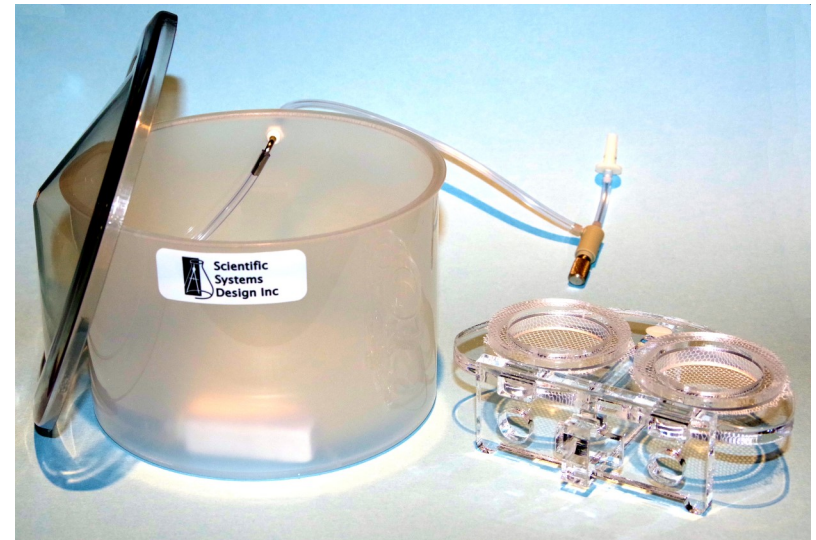
Above: BSK5-2 Brain slice keeper with rings and net in place and with purpose designed container with lid to side. A needle valve is used to control the flow of oxygen mixture to the air-stone. Below: View of two-ring manifold.
