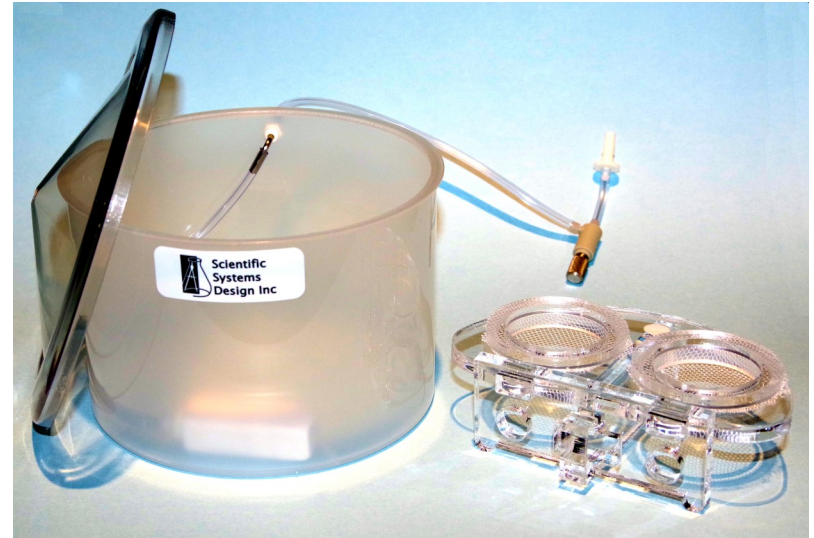
Above: BSK4 Brain slice keeper with rings and net in place and with lid in place (inset). A needle valve is used to control the flow of oxygen mixture to the ceramic air-stone. Below: View of two-ring manifold.
