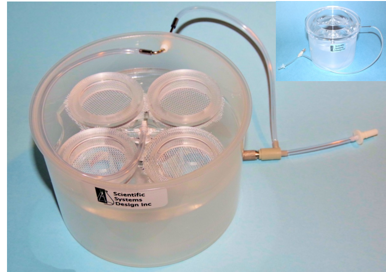
BSK4 Brain slice keeper with rings and net in place and with lid in place (inset). A needle valve is used to control the flow of oxygen mixture to the ceramic bubbler.
