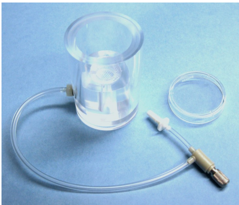
BSK2 Components - chamber with insert in place, needle valve gas flow regulator and lid.
