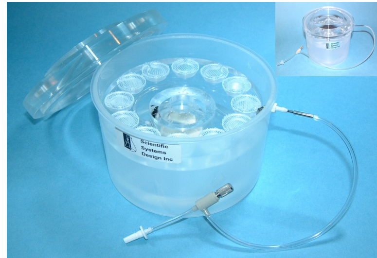
BSK12 Brain slice keeper with rings and net in place and with lid in place (inset). A needle valve is used to control the flow of oxygen mixture to the ceramic bubbler.
