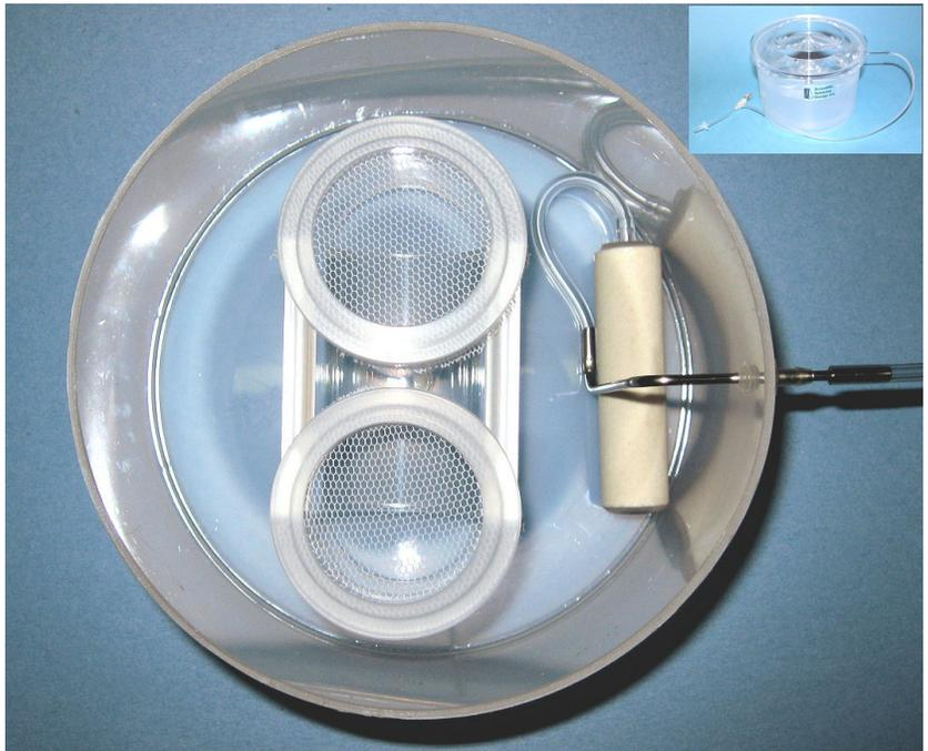
***BSK5-2 viewed from above. Brain slice keeper with rings and net in place and with lid in place (inset). An included needle valve is used to control the flow of oxygen mixture to the ceramic bubbler.***
