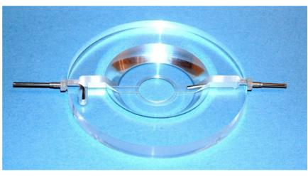
SPECIFICATIONS Size: 100mm diameter X 10mm Material: Clear acrylic Coverslip base: 22mm X 150um . Inlet tube: Stainless steel tube, 1.8 mm O.D. Exit tube: As for inlet tube Dead space: Min. capacity of pool formed above
