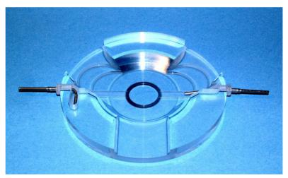
the central coverslip base [3] so that the perfusion solution forms a pool around the preparation whilst being refreshed by virtue of the inlet and exit ports.
