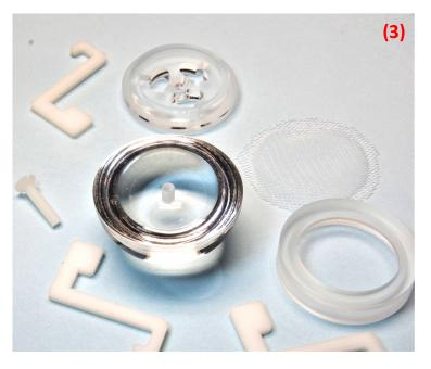
(3) Discard the nylon netting. Clean the remaining seven separate components as necessary in distilled water or immerse all parts in 10% diluted 30 or 20 Vols hydrogen peroxide (H2O2) over-night. Rinse in distilled water.
