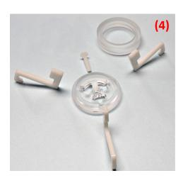
(4) After washing in distilled water dry all components at room temperature
