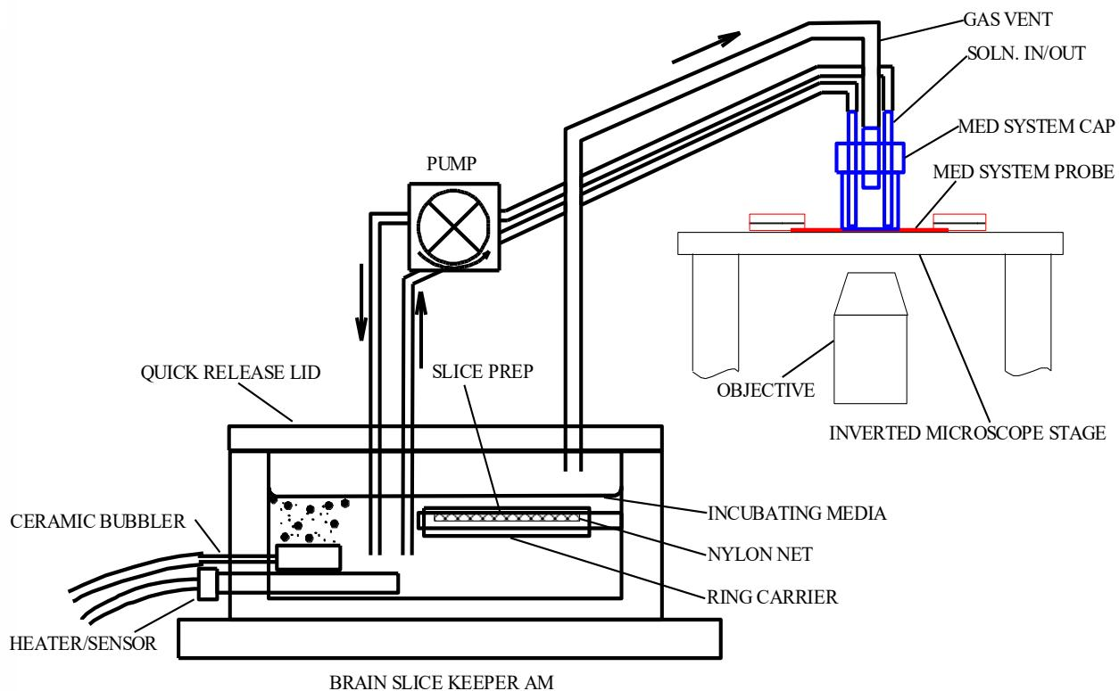
Pipes and tubes should be as short as possible and arranged to be well thermally insulated to minimise the temperature drop from the incubating area to the recording area. The PTC03 temperature controller is electrically quiet and should not produce any interference in recordings. Peristaltic pumps may need to be grounded and shielded and kept at a distance from the recording area.
