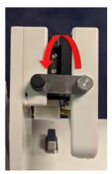
1. Remove thumbscrew that is on the right side of the transportation fixture. You do not need to remove anything on the left side (leave as is).
