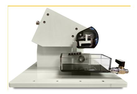
The VF-510-0Z tissue slicer model is the latest version of our flagship product in the Compresstome<sup>®</sup> slicer family. With patented Auto Zero-Z<sup>®</sup> technology, the VF-510-0Z is fully automated to section both fixed and live tissues with a thickness range of  $4 \mu m^*$  to 1000  $\mu m$  and an adjustable precision of  $1 \mu m$ .
