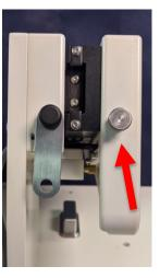
2. After removing the thumbscrew, the transportation fixture will fall shown in the picture above. Place the thumbscrew back into the machine so that it does not get lost and that you can reattach the transportation fixture for any future shipments.
