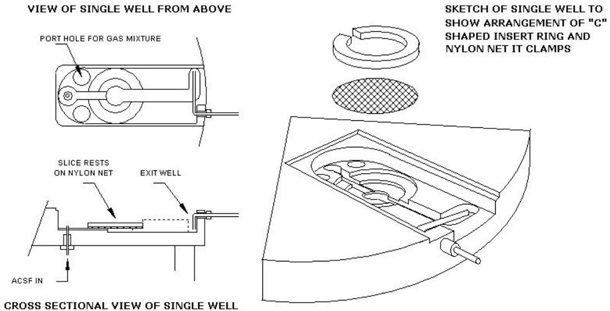
stainless steel. (Steel should either be coated with an anti-corrosive film or nickel electroplated). The four 90 degree or the three 120 degree pattern fixing holes in the base can be used to mount small magnetic bases if a steel or special magnetic stainless steel table is used as a base. The base-plate must not become distorted through securing on to an uneven base, nor should nuts and bolts be over tightened in the holes provided.
